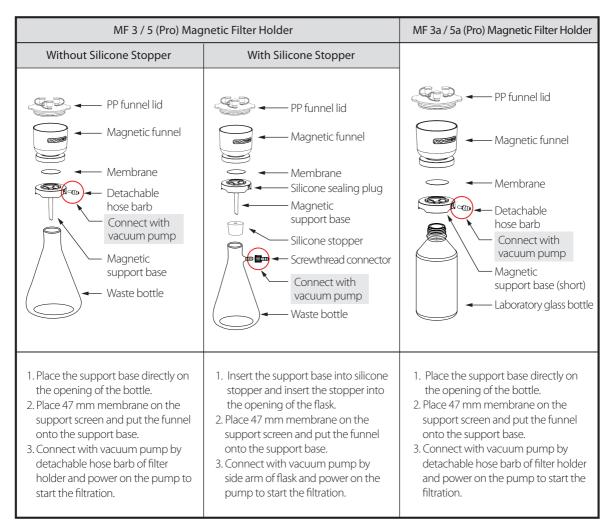
• If a funnel lid is necessary during filtration, open a cap and insert a syringe filter for venting.
